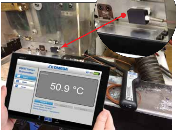
Figure 1: UWBT-TC-UST transmitter monitoring mold temperature
