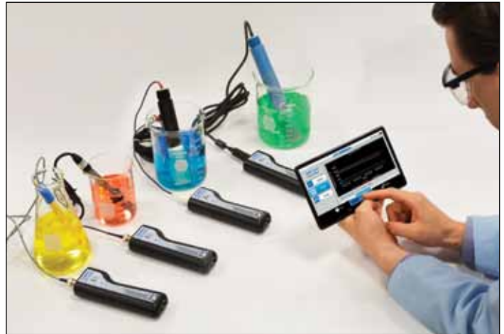
Figure 2: Four UWBT-PH transmitters connected to one tablet
