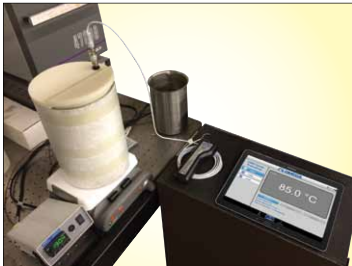
Figure 1: UWBT-RTD-TB shown recording temperature data from a PR-31 RTD probe
