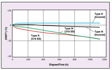
Figure 1. Drift of 3 mm diameter stainless steel sheathed and Inconel 600 sheathed type K and Nicrosil vs. Nisil thermocouples in 1200°C in vacuum. The dips in the drift curve are the result of the "in-place inhomogeneity test" where the samples were extracted from the furnace by 5 cm.
