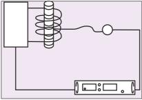
Figure 3: Controlling induction treating of automotive crankshafts.
