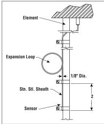
High Limit Controls — Electronic high limit controls can be mounted on the heater chamber with an overheat thermocouple welded to heating element sheath inside the chamber. This arrangement provides protection by shutting down the heater at a predetermined element sheath temperature. Option also available with thermocouple only, welded or clamped to heater element sheath as shown above.
