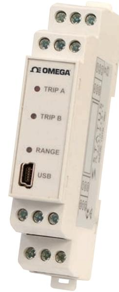
The TXDIN1600s is a “smart” powered bridge amplifier for use with strain gauges or load cell signals. The product has a built in capability to scale the input signal to a process value while the output stage offers either voltage, bipolar voltage or active / passive current re-transmission signals.
