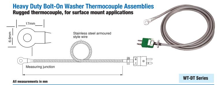
Rugged thermocouple, for surface mount applications. Rated to 480°C, has a SS mounting washer with dimensions of 17.3 mm O.D., with a 6.6 mm mounting hole. Attached to the mounting surface: 2 m of SS flexible armour cable with stripped wire ends. Armour cable has 7.0 mm O.D., with 1.8 mm washer thickness. Standard thermocouple plugs are available for cold-end termination.
