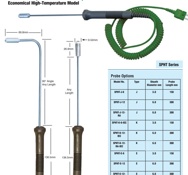
The spring mounted thermocouple tip ensures optimum surface contact and a fast response time. The SPHT comes with a mini plug which makes the probe ideal for use with handheld thermocouple thermometers. The sensor head is 9.5 mm diameter and 27 mm long, mounted on a 3 mm diameter stem for 150 mm long probes and 6 mm diameter for 300 mm.
