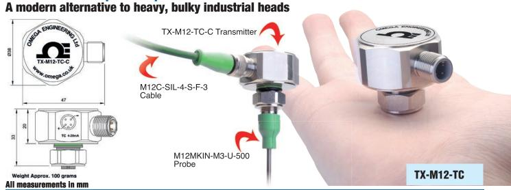
Omega's TXM12 series transmitters offer improved performance over conventional in-head transmitters yet are a fraction of their size and weight. Integral M12 connectors maintain IP67 protection and connection integrity whilst allowing for a quick and simple change of sensor. The TX-M12-TC-C transmitter is ideal for use with Omega's M12 range of thermocouple probes, which connect directly to the TXM12 sensor input.
