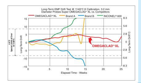
Super OMEGACLAD® XL Probes are an excellent choice for high temperature measurement. They provide very low drift at high temperatures as compared to conventional Inconel and Stainless Steel sheathed probes. They are available in both K and N thermocouple calibrations. Omega offers probes in a variety of styles.
