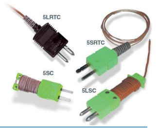
All models are available with 1 or 2 metre wire lengths and 3 types of wire insulation: Kapton and PFA provide good protection against moisture and abrasion resistance and are rated for maximum service temperatures of 315°C and 260°C respectively providing at the same time a fast response to temperature changes. Glass Braid is rated for a maximum service temperature of 480°C. Wire diameters of 0.08, 0.13, 0.25, 0.5 and 0.8mm are available.
