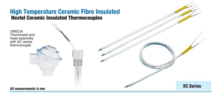
OMEGA® Nextel Ceramic Insulated Thermocouples are easy-to-use precise temperature elements manufactured to meet the highest industry standards. The Nextel ceramic insulation is rated for 1200°C continuous use, or 1425°C short term. These highly versatile elements are the ideal solution for many high temperature applications. Combined with OMEGA's stock thermowells and industrial heads, a complete head and well assembly can be quickly assembled for fast delivery.
