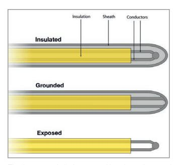
The thermocouple in the exposed junction style protrudes out of the tip of the sheath and is exposed to the surrounding environment. This type offers the fastest response time, but is limited in use to noncorrosive and non-pressurized applications. See the illustration above for a full discussion of junction types. The sheath insulation is sealed where the junction extends to prevent penetration of moisture or gas which could cause errors.
