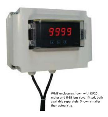
The WME housing provides a wall mounting option for 1/8 DIN panel meters and controllers with a maximum depth of 110 mm. Access for wiring is provided by cable glands mounted on the bottom of the housing. The WME housing provides IP65 protection and the SPC18 clear front lens cover is also available for use with instruments that do not have an IP65 front panel/lens rating (such as the DP20) to ensure complete IP65 sealing of the instrument.
